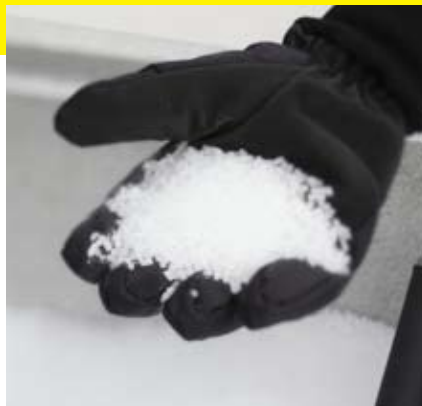
Machine is filled with 3 mm dry ice pellets.
