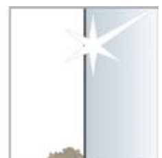
In the process the dry ice sublimates, leaving only the coating that has been removed behind, which can be simply swept from the floor.
