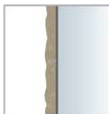
Dry ice cleaning works on the principle of 3mm pellets of dry ice being propelled at great speed onto a contaminated surface.
